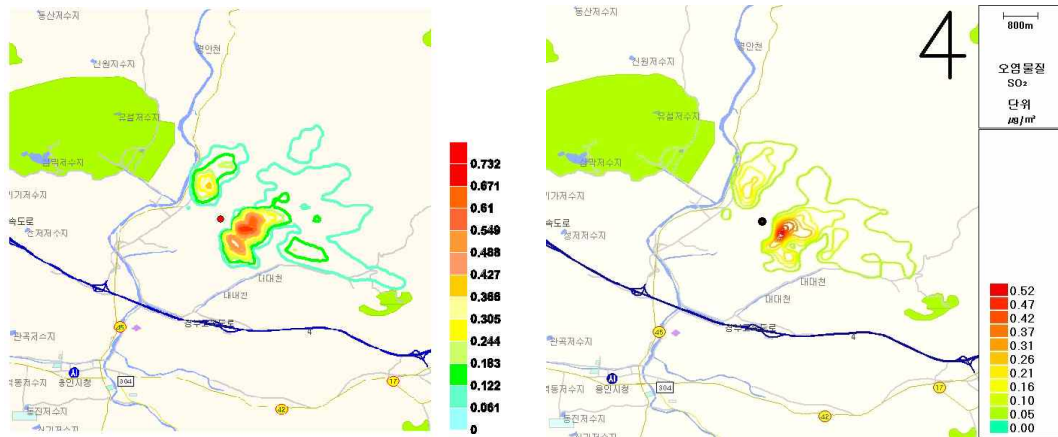
Fig. 41. Comparison of annual average \text{SO}_2 concentration predicted by PUFF model with Gaussian model.
